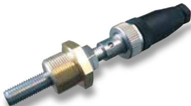
ZRPM1 RPM Counter Inductive proximity sensor, c/w female connector M12 4 pin, IP67, field attachable, ring nut reduction M18 x 1. Power Supply: 12/24 VDC
