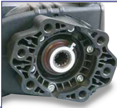
SAE J744-C Spline Shaft 14T 12/24 DP Hydraulic Drive.
