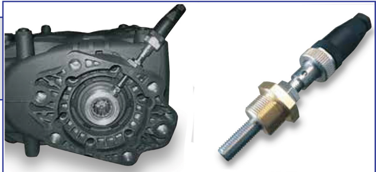
ZRPM1 RPM Counter Inductive proximity sensor, c/w female connector M12 4 pin, IP67, field attachable, ring nut reduction M18 x 1. Power Supply: 12/24 VDC
