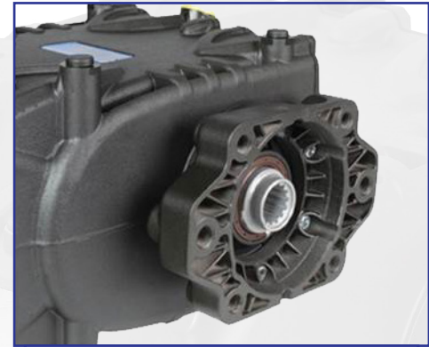
SAE-C 2/4 F 14 tooth 12/24DP hydraulic drive
