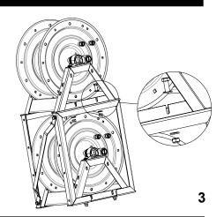
3) Bolt your second hose reel the ASSEMBLY FRAME/BRACE/ HOSE REEL assembly. Again, use (4) M12 nuts and bolts and (8) M12 washers.
