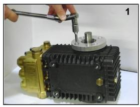
1. Remove four bolts from side cover. Mount adapter plate to pump. Apply Loctite 243 thread locker to bolts and torque to 14.7 Ft. Lbs.
