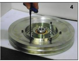
Mount pulley(s) to clutch assembly and apply Loctite 243 thread locker to bolts. Torque bolts to 8.8 Ft. Lbs.
