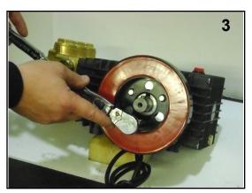
3. Mount coil to adapter plate. Torque bolts to 7.3 Ft. Lbs.
