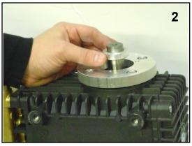
2. Install spacer ring on shaft.
