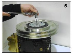
Apply anti-seize lubricant to pump shaft. Slide pulley/clutch assembly onto pump. Fasten using bolt with washer. Apply Loctite 243 thread locker to bolt and torque to 8.8 Ft. Lbs.
