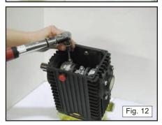
9) Install rear crankcase cover respecting O-ring seal. Torque bolts to specifications. Fig. 13.
