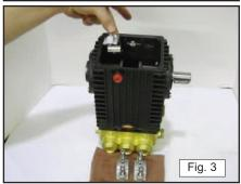
3) Remove connecting rod cap bolts with 6 mm hex wrench, respecting position and orientation of each cap. Position connecting rod/plunger guides fully into crankcase to allow clearance of crankshaft removal. Fig. 2 and 3.
