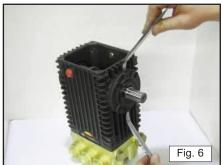
Remove crankshaft out crankcase side cover hole and reassemble shaft position to opposite side. Fig. 8.
