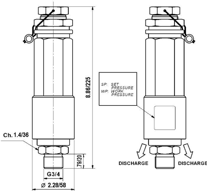
**ATTENTION:** Safety valves are set 15 to 20% above the maximum operating pressure of the system. The real cracking pressure of a SV3/300 (for example) is 4,350 PSI plus 20% = 5,220 PSI.
