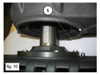
Fasten the gear housing with the 6 M8 x 50 screws and tighten the latter with a torque wrench (Fig. 11 and 12) as indicated in section 9.
