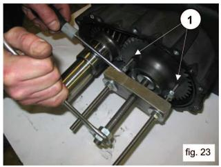
Remove the pinion using a percussion extractor on the M12 hole (Fig 24). Loosen the gear housing screws and remove the housing screws and remove the housing (Fig. 25).
