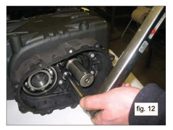
Insert the crown into the pump shaft, apply the washer and use the wrench (Fig. 13) to tighten the screws to the torque level indicated in section 9. Fix the two Ø5 pins to the gear housing (Fig. 14, position 1).
