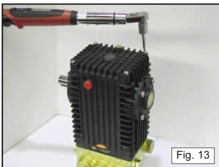
8) Install each connecting rod cap back to original place. Fig. 3. Torque bolts to specifications. Fig. 12. Rotate crankshaft to assure smooth operation.
